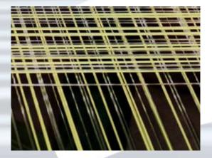
The stitch-bonded, multi-axial construction of V2's non-crimp fabrics prevents the degradation of fiber strength that occurs with conventional woven fabrics. Straight line construction promotes optimal physical properties of
